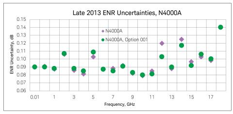
Figure 2. Example ENR versus frequency for the N4000A model.
