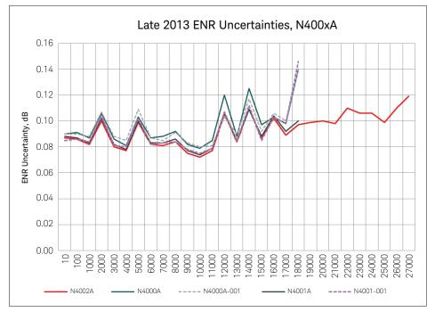
Figure 4. Characteristic ENR plot versus cardinal frequency points.
