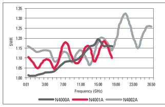
Figure 1. Characteristic SWR at 23°C
